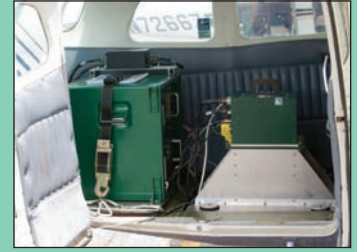
LIDAR equipment mounted in airplane.
